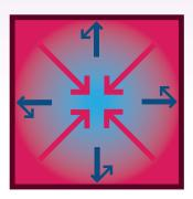
In conventional dehydration, heat flows from the outside to the inside. This closes the surface pores and keeps the evaporating moisture from escaping. Drying time is extended, usually causing material damage and an altered appearance.
